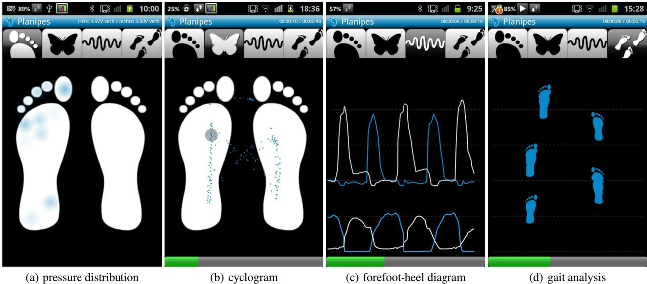
**Figure 4.** Screenshots of the Planipes application running on an Android smartphone. Using four different screens (pressure distribution, cyclogram, forefoot-heel diagram, and gait analysis) the incoming sensor data can be visualized according to the specific use case.
