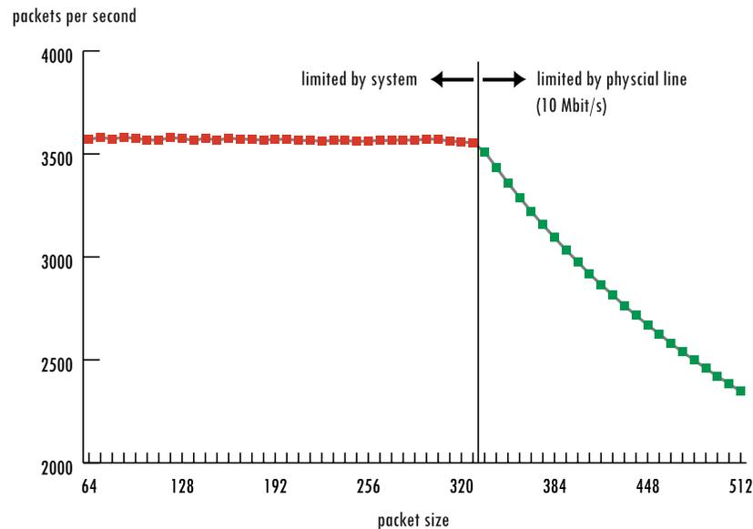
**Figure 1-2: Measured throughput in packets per second for different packet sizes**
