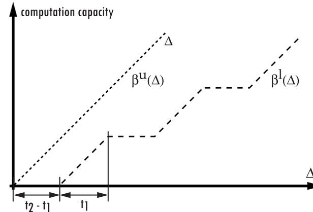
Figure 6-3: Lower and upper service curve for RNOS on target system
