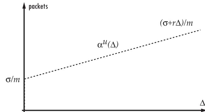
**Figure 2-4:  $(\sigma, \rho)$  model as upper arrival curve**
