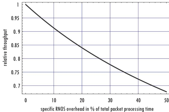
**Figure 5-16: Impact of Overhead on Throughput**
