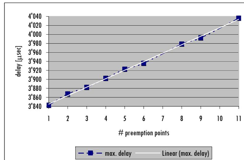
**Figure 6-11: Maximum delay vs. number of preemption points**
