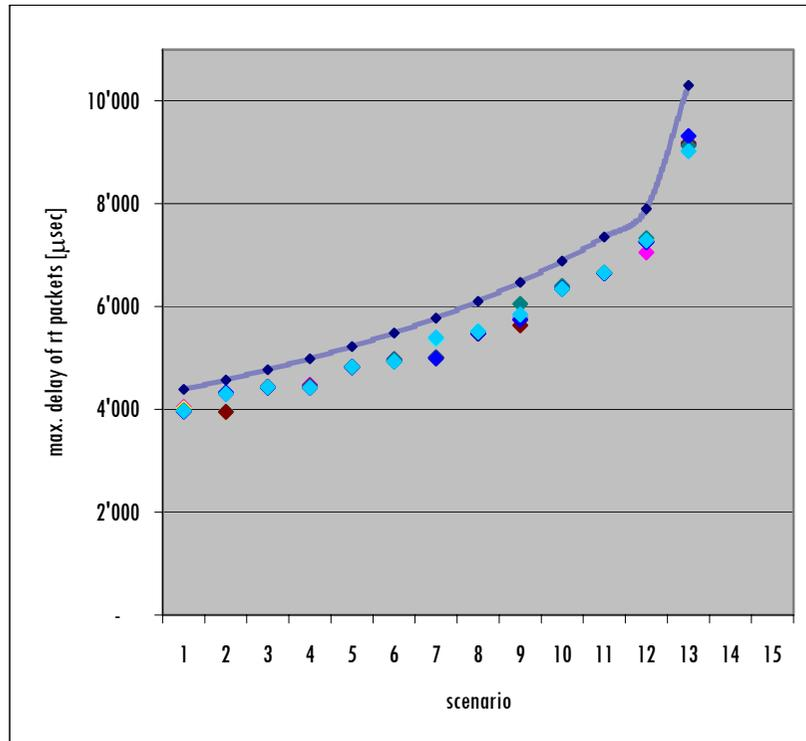
Figure 6-18: Maximum delay measurement (2 preemption points, real-time flow)
