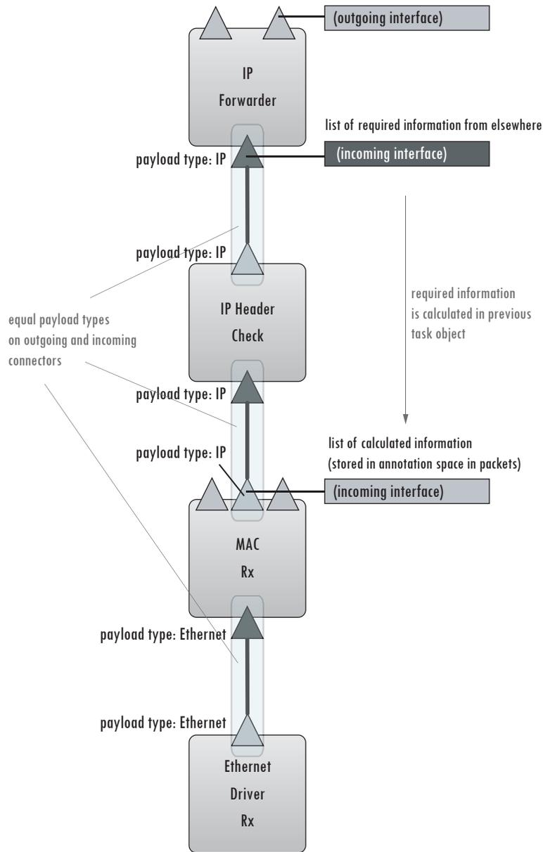
**Figure 5-2: Connectors must match in payload type and required annotations**
