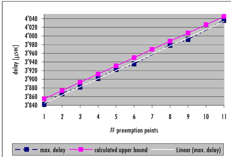
**Figure 6-13: Measured max. and calculated upper bound of delay**
