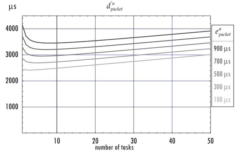
**Figure 5-21: Upper bound of delay for highest priority packet**
