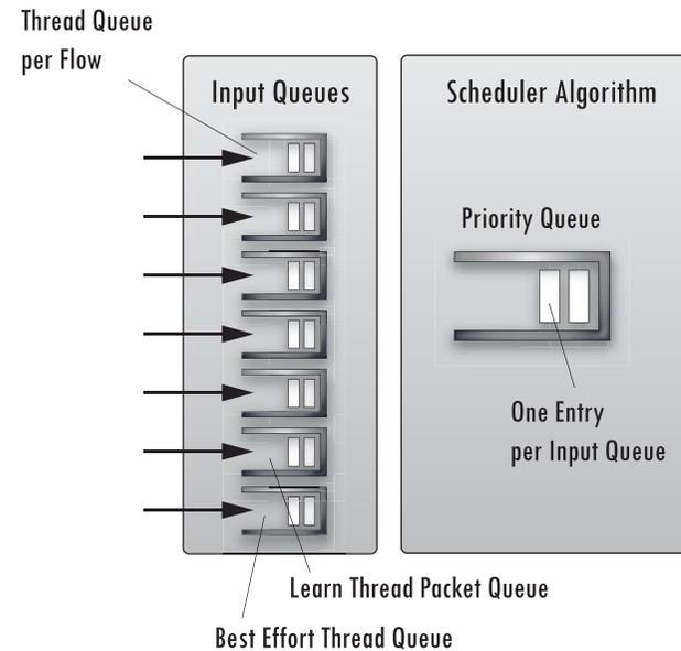
**Figure 5-10: Scheduler Architecture with EDF Algorithm**
