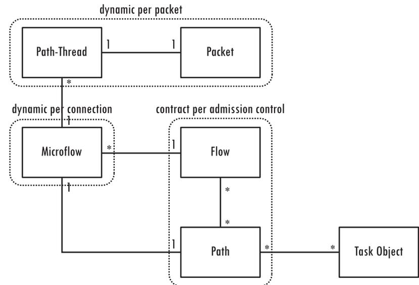
Figure 5-8: Object Relation Diagram with Microflow Object
