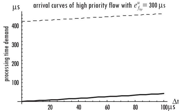
Figure 5-26: Example arrival curves of high-priority flow
