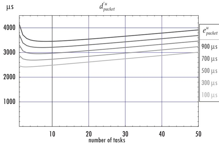
**Figure 5-28: Upper bound for delay for packets of highest priority flow**
