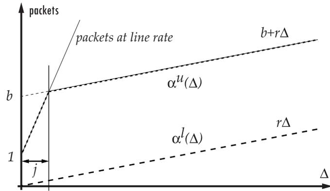
Figure 2-7: Arrival curves for constant rate packet source with network jitter
