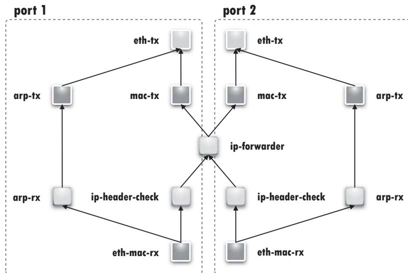
**Figure 4-2: Possible implementation model of the two port router**
