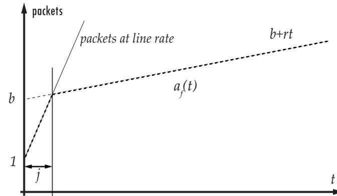
Figure 2-6: Arrival function for constant rate packet source with network jitter
