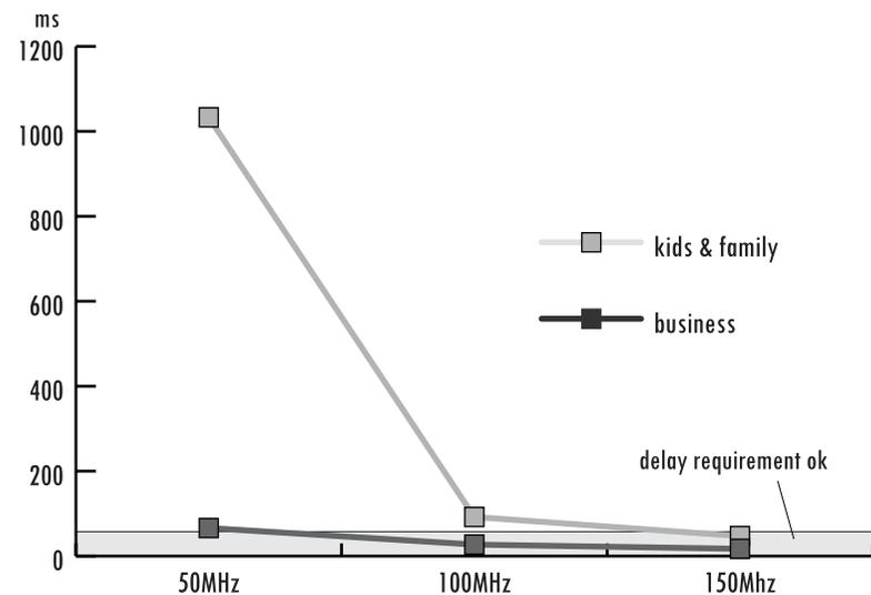
**Figure 3-9: Delay of kids & family and business flow for different CPU clock speeds**
