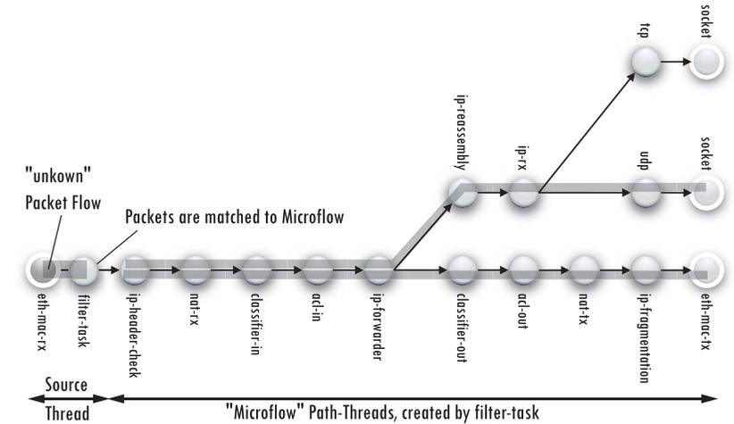
**Figure 5-9: Source Thread creates Path-Threads**
