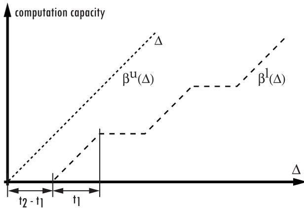
Figure 2-15: Upper and lower service curves for a CPU resource
