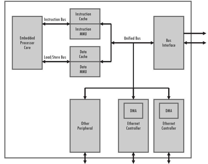
**Figure 1-1: Block Diagram of a typical Embedded Communication Controller**
