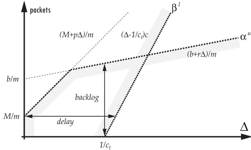
**Figure 3-1: Bounds on delay and backlog**
