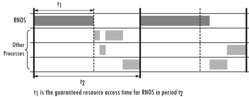
**Figure 5-13: RNOS running on RTOS as a process**
