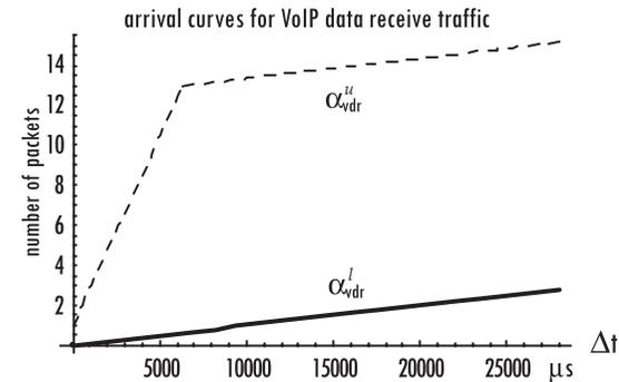
**Figure 3-7: Arrival curves for VoIP data receive flow**
