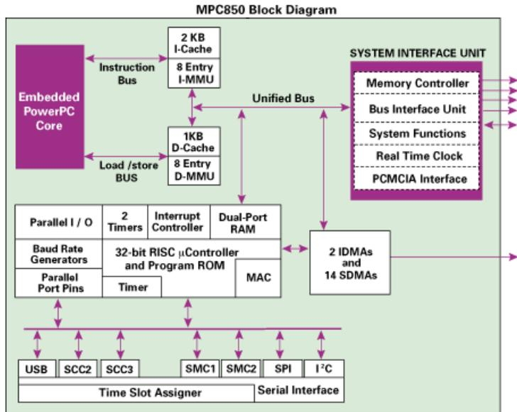
Figure 6-1: Block Diagram of Embedded Controller
