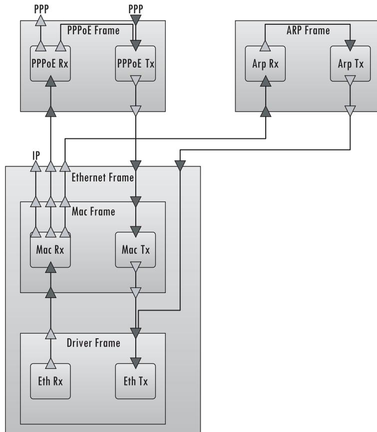
**Figure 5-4: Link Layer with Task Frames**
