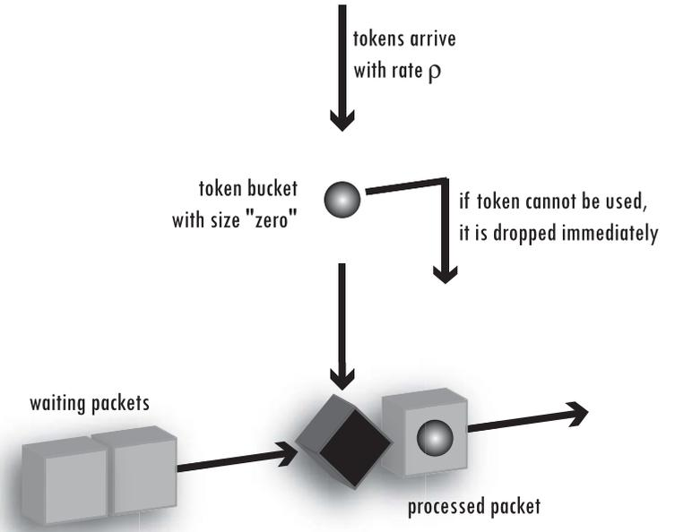
**Figure 3-2: Physical processing model**
