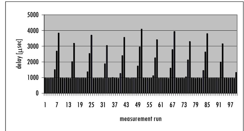
**Figure 6-5: Delay measurement result (11 preemption points)**
