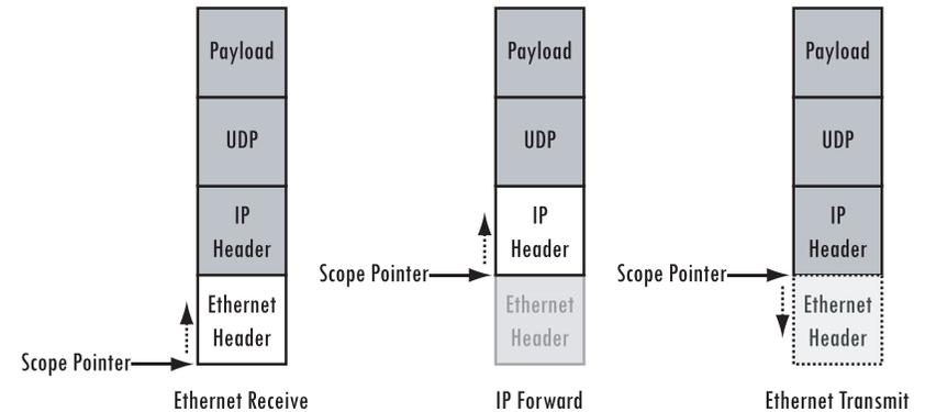
**Figure 5-7: Scope on packet data**
