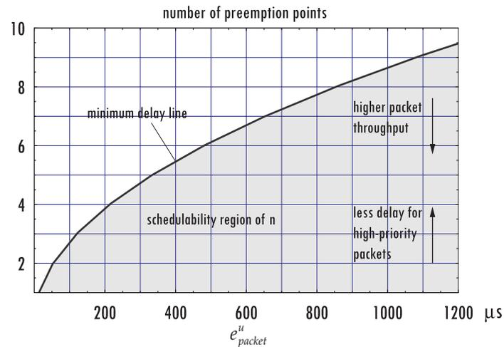
Figure 5-22: Feasible number of preemption points, depending on  $e_{packet}^u$
