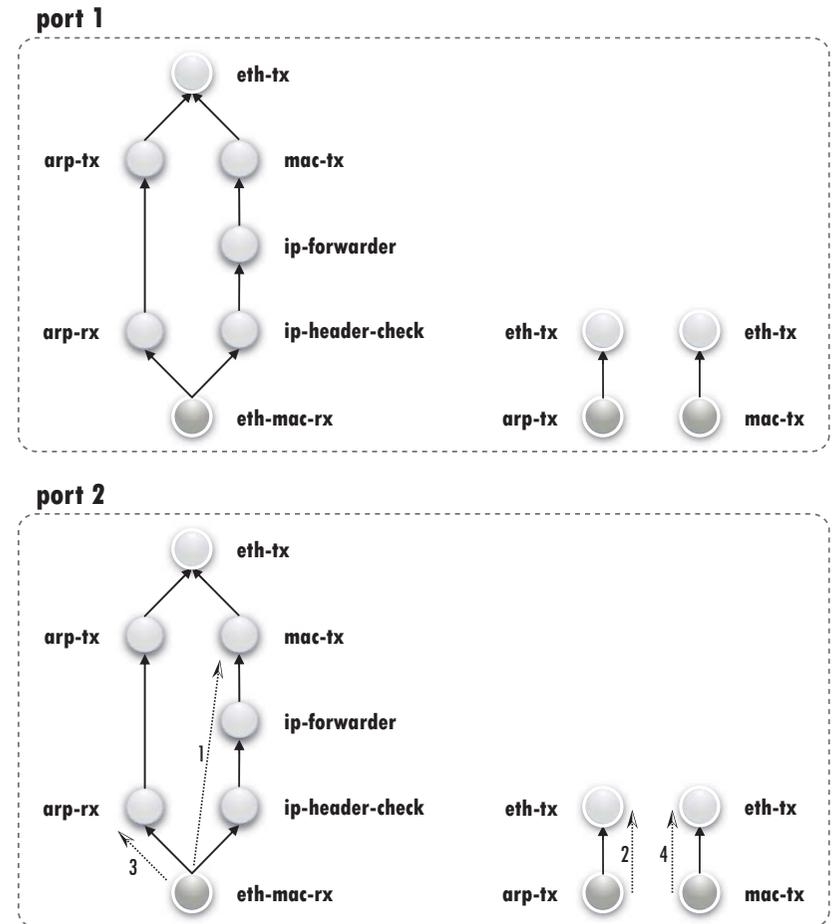
Figure 4-1: Model of two port router
