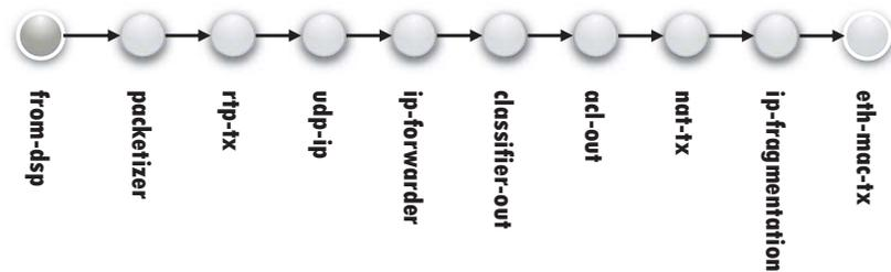
Figure 2-11: Task graph from DSP to Ethernet
