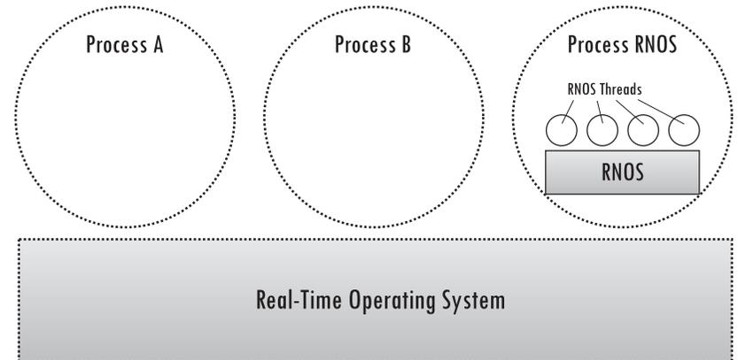
**Figure 5-12: RNOS running in an RTOS process**
