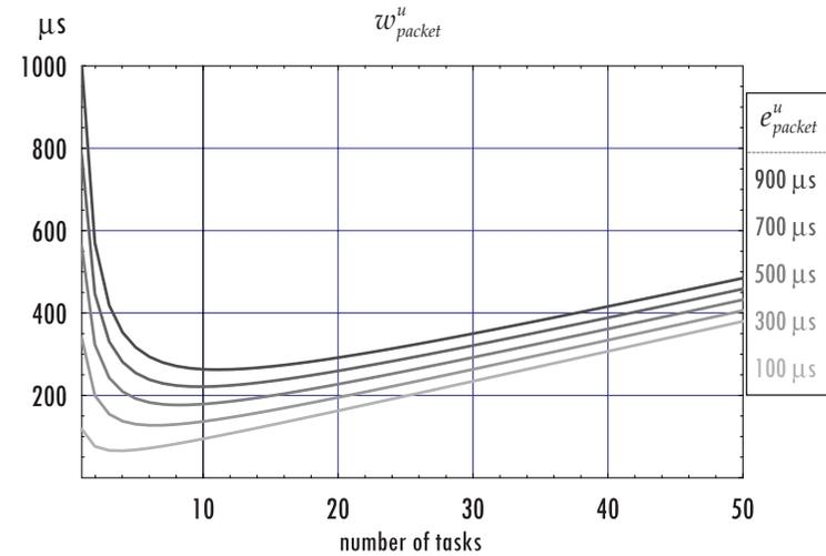
Figure 5-19: Upper bounds for waiting times for a highest priority packet
