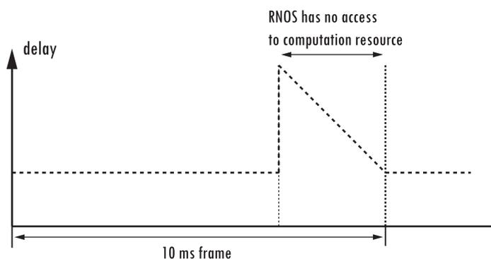
Figure 6-7: Delay of single packet
