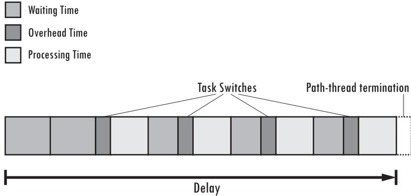
**Figure 5-20: Worst-case overhead time for a highest-priority packet**
