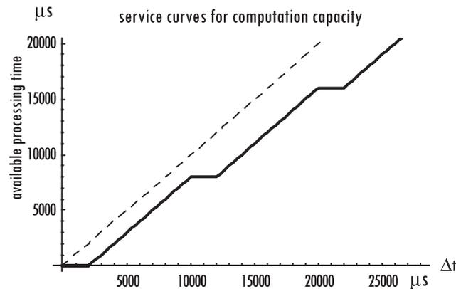
Figure 5-27: Service curves of processing resource
