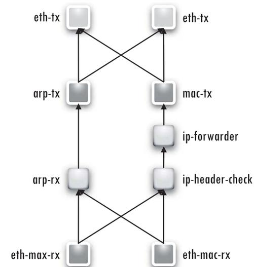
**Figure 4-3: Another implementation model of the two port router**
