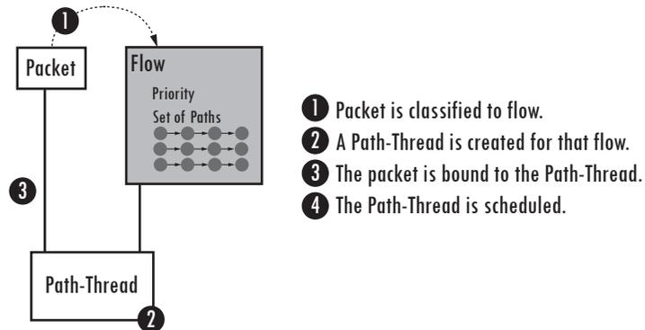
**Figure 4-5: Packet and Path-Thread**
