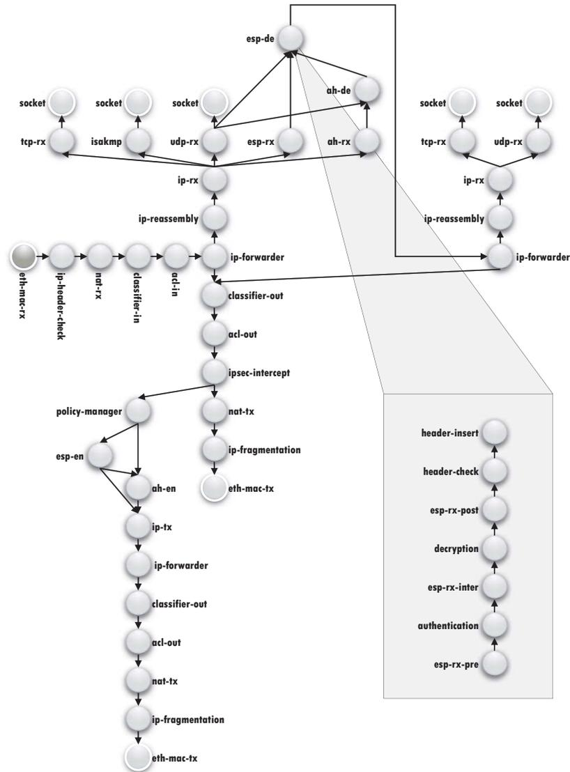
Figure 2-12: Simplified task graph for packet reception with IPsec support
