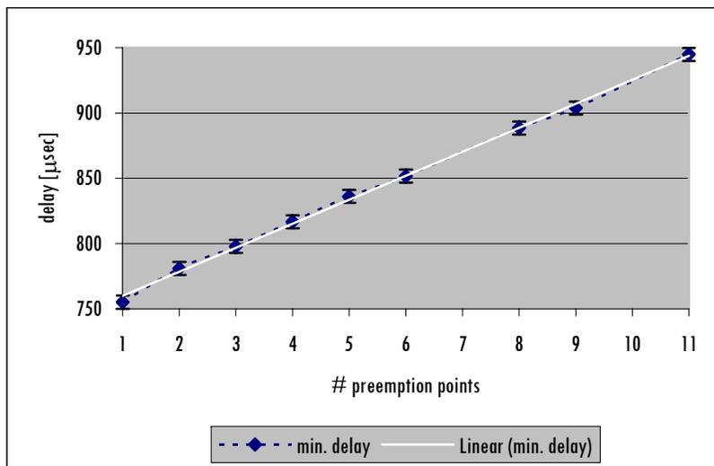
**Figure 6-9: Minimum delay vs. number of preemption points**
