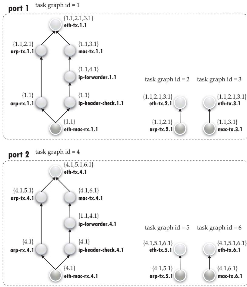
Figure 4-4: Task graph of a two port router annotated with instance information
