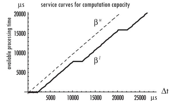
**Figure 3-8: Service curves for computation capacity**
