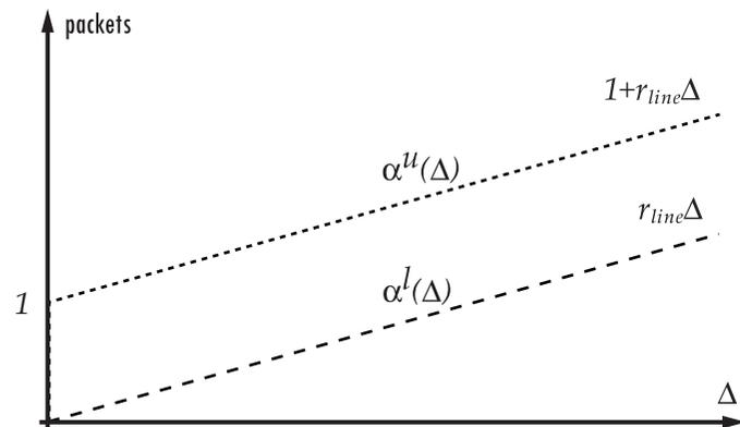
Figure 2-8: Arrival Curves for smallest packets back-to-back on line
