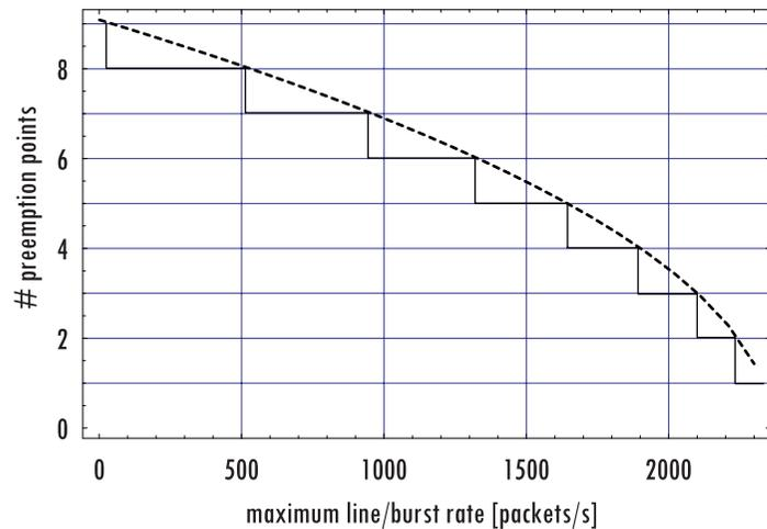
**Figure 6-15: Maximum number of feasible preemption points for a long path**
