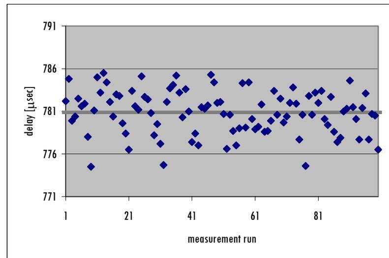
Figure 6-8: Minimum delay measurement (2 preemption points)
