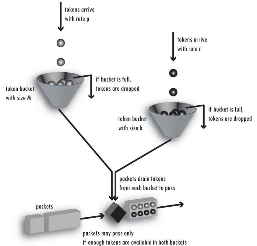
**Figure 2-3: Dual Token Bucket for TSpec**
