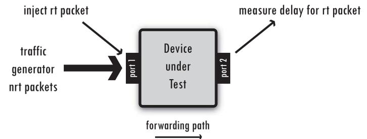
**Figure 6-16: Measurement setup with one rt-flow and multiple nrt-flows**
