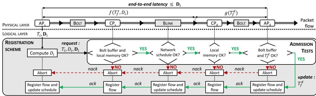
Figure 2. Steps and components involved when registering a new flow in DRP. Given a request for a new flow  $F_i = (s_i, d_i, T_i, D_i)$ , the source node's AP computes the flow's network deadline  $D_i$ . Then, all components successively verify using specific admission tests whether they can admit the new flow. DRP registers a flow only if all admission tests succeed, which triggers changes in the runtime operation (i.e., schedule) of some components.
