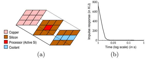
**Figure 12: (a) Schematic of the general thermal model considered, and (b) its impulse response.**
