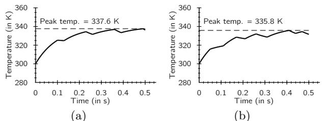
Figure 2: Temperature evolution for power traces shown in (a) Figure 1(a), and (b) Figure 1(b) of Example 1
