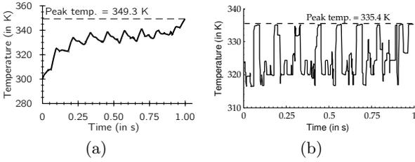
**Figure 11: Temperature plot for flipped PVC trace for (a) the Fourier heat model, and (b) the thermal model with active cooling.**
