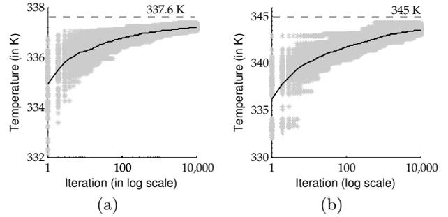
**Figure 5: A plot of the peak temperature noted during random simulations for (a) Example 1 and (b) Example 2.**
