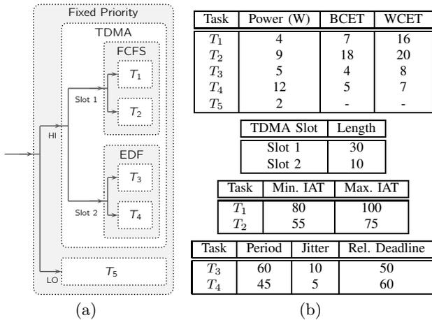
Figure 8: (a) Hierarchical scheduling of tasks, and (b) Task parameters. All times shown are in ms.
