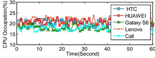
Figure 22: CPU utilization.
