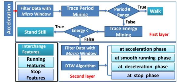
Figure 6: Work flow of acceleration feature extraction.
