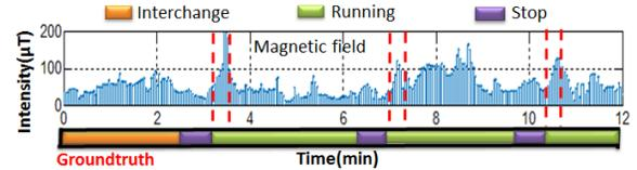
**Figure 3: Magnetic field trace of a metro trip.**
