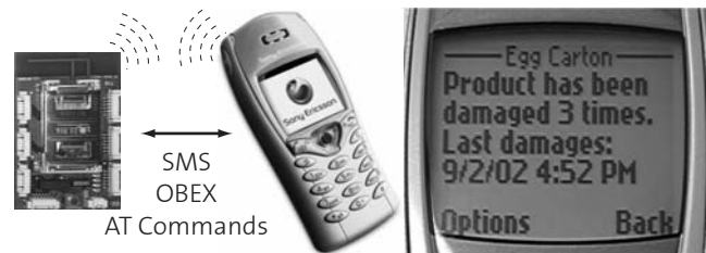
Figure 1: Product monitoring using BTnodes as smart tags and SMS via mobile phones.
