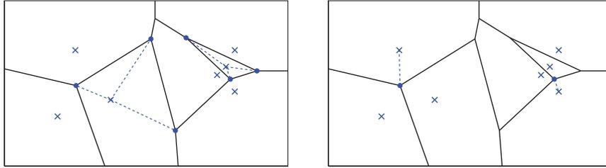
**Fig. 2** Illustration of the Voronoi mutation: crosses denote sensor nodes, circles denote Voronoi vertices. The relative probabilities to delete (left) and add (right) a sensor node are depicted exemplary: on the left, the point to the right is more likely to be removed; on the right, the point to the left is more likely to be added.
