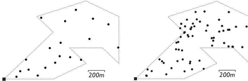
**Fig. 3** Two examples for evolved node placements for the same area of interest outlined by a polygon. Nodes are marked by circles and the sink is indicated by a square. Both solutions are part of the respective Pareto front approximations found with the parameters  $\kappa = 1.0$  and  $\rho = 1:3$ . The left solution corresponds to an objective vector of  $(f_1, f_2) = (18, 0.5827)$  while the network on the right has objective values  $(f_1, f_2) = (61, 0.0016)$ .
