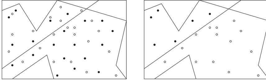
**Fig. 1** Illustration of the crossover: (left) sensor node positions of the two parents (filled/empty); (right) first child, containing all positions from the first parent lying above the line and all positions from the second parent lying below the line.
