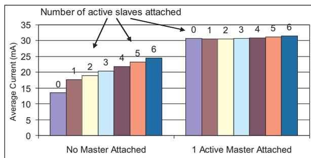
**Figure 4. Active links; left cluster: 0 to 6 slaves attached (piconet); right cluster: 0 to 6 slaves plus 1 master (scatternet).**
