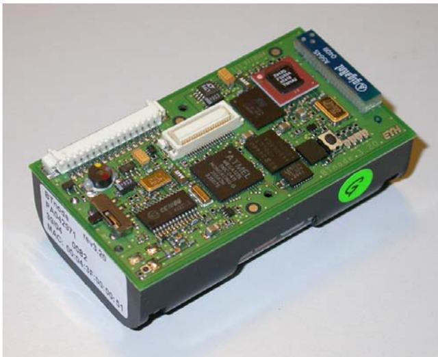
The BTnode rev3 has been designed with two radios and power conversion and distribution systems. The low-power radio is the same as used on the Berkeley Mica2 Motes, making the BTnode rev3 a twin of both the Mote and the old BTnode rev2. Both radios can be operated simultaneously or be independently
