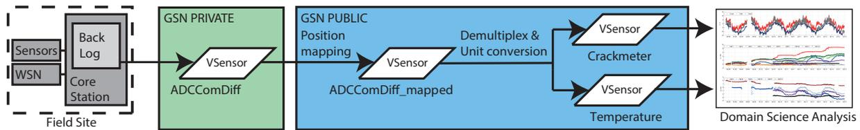
**Figure 1:** Data from the field sites is stored in unmodified form in the primary instance of the GSN data management server. After mapping of metadata and value conversion it is stored as secondary data in the public instance of GSN from where it is accessible by various tools.
