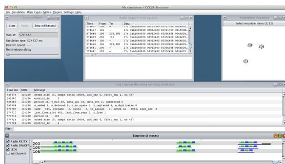
(a) Cooja with visualizations of a simulation. The *Timeline* plugin at the very bottom displays packet transmissions and receptions in the network
