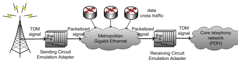
**Fig. 1. – Circuit emulation over MAN Gigabit Ethernet: Connecting a base station to the core PDH network requires packetizing the base station's E1/T1 PDH signal into Ethernet frames and synchronization across the Ethernet. This synchronization is difficult since the fill state of the receiver's play-out buffer is impacted by both Ethernet dynamics and the difference in frame sending and buffer read-out frequency.**
