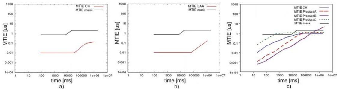
**Fig. 4. – Sample results of CEA’s synchronization performance in software simulation and testbed: a) MTIE for Convex Hull in software simulation; b) MTIE for Linear Adaptive Approximation in software simulation; c) Resulting MTIE for Convex Hull, Product A, Product B in the testbed.**
