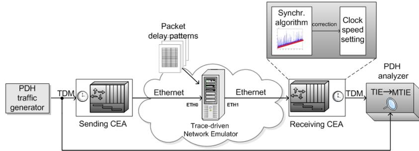
**Fig. 3. – Testbed to evaluate the synchronization performance of CEAs: At the sender’s side a fully-fledged hardware implementation of a CEA packetizes E1/T1 PDH signal into Ethernet frames. Ethernet frames go through a network emulator. At the receiver’s side a peer CEA reassembles PDH signal and adjusts the play-out rate. The network emulator is driven by frame delay traces from real networks.**
