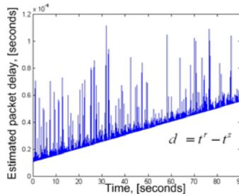
**Fig. 2. – Illustration of the effect of the clock skew on end-to-end frame delay estimated from sender and receiver timestamps: minimal end-to-end delay has an increasing trend due to difference in frame sending and buffer read-out frequency.**
