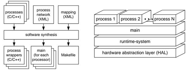
Fig. 5. Software synthesis (left) and the structure of the resulting software stack for a single processor (right).
