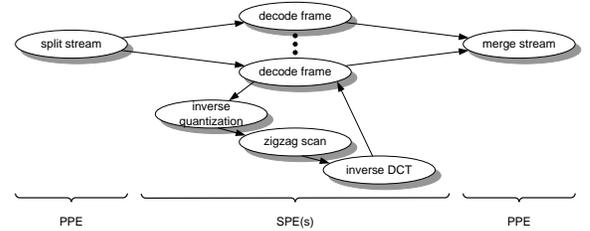
Fig. 9. KPN of the MJPEG decoder. The lower part of the KPN indicates the structure of the fine-grained implementation.
