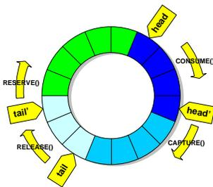
Fig. 2. Implementation of windowed FIFO.
