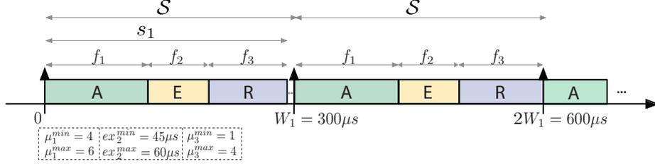
Figure 2: Two consecutive executions of superblock set  $S$  (worst-case): The WCRT of  $S$  is equal to  $W_j$  due to interference over shared resources.
