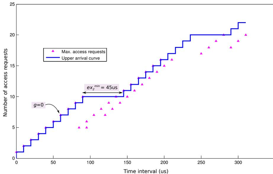
Figure 3: Upper arrival curve with constructing tuples for superblock set  $S$  ( $C = 10\mu s$ ,  $g = 0\mu s$ )
