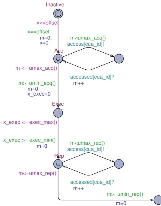
Figure 6: Superblock - Single execution starting `offset` time units after the beginning of the arbitration cycle.
