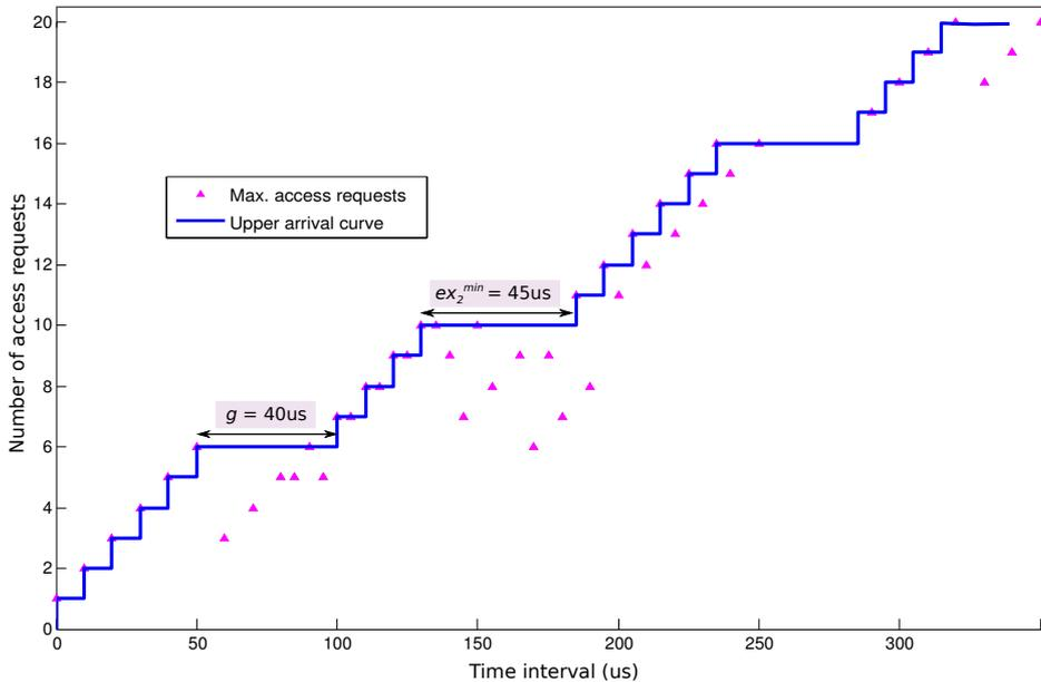
Figure 4: Upper arrival curve with constructing tuples for superblock set  $S$  ( $C = 10\mu s$ ,  $g = 40\mu s$ )
