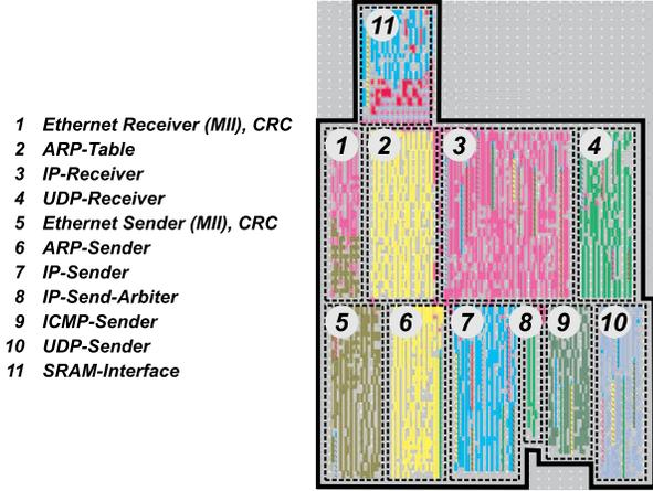
Figure 8. Floorplan of the minimal IP stack.
