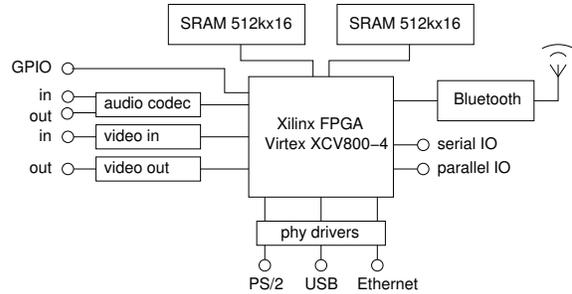
Figure 5. Block diagram of the WURM prototyping platform.
