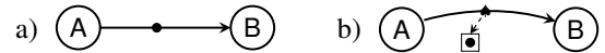
Figure 2: Two KPN approaches: a) Classic process network; b) Process network with shared memory blocks. The spade represents an access token linked to a memory block with the "classic" token from before.
