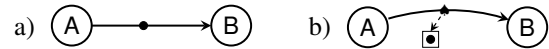
Figure 2: Two KPN approaches: a) Classic process network; b) Process network with shared memory blocks. The spade represents an access token linked to a memory block with the "classic" token from before.
