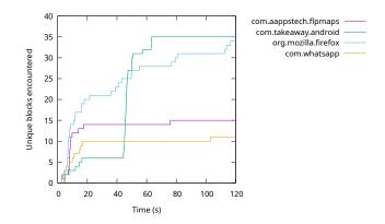
Fig. 6. Unique blocks encountered while running a few apps from Google Play while providing a random input every 100 ms for 2 minutes using Monkey.
