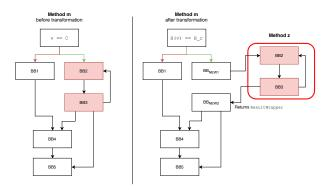
**Fig. 2.** Comparison of an example of a control flow graph before and after transformation. Basic blocks (BB) with a red background represent the basic blocks whose instructions can be extracted to a separate class and encrypted.
