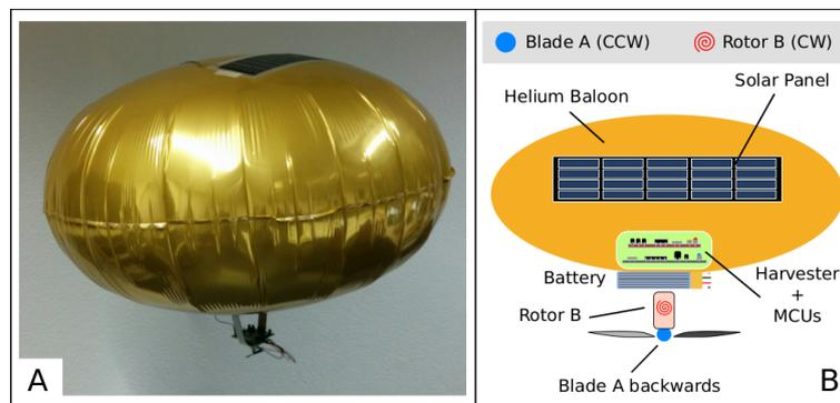
Figure 1: Slightly heavier-than-air Vehicle
