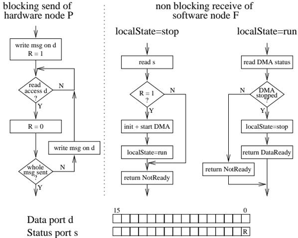
**Figure 7. Interface refinement for channel B**
