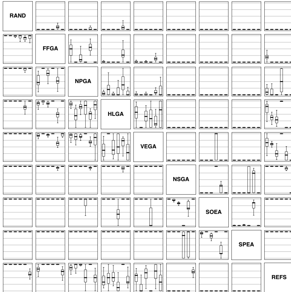
Figure 7: Box plots based on the \mathcal{C} metric. Each rectangle contains six box plots representing the distribution of the \mathcal{C} values for a certain ordered pair of algorithms; the leftmost box plot relates to \mathcal{T}_1 , the rightmost to \mathcal{T}_6 . The scale is 0 at the bottom and 1 at the top per rectangle. Furthermore, each rectangle refers to algorithm A associated with the corresponding row and algorithm B associated with the corresponding column and gives the fraction of B covered by A ( \mathcal{C}(A, B) ). Consider, for instance, the top right box, which represents the fraction of solutions in the reference sets covered by the nondominated sets produced by the random search algorithm. For each test function and each optimization run, RAND covered 0% of the corresponding reference set.
