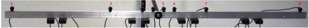
Figure 3: Microphone array consisting of eight microphones mounted on a bracket. The black boxes under the bracket are the microphone preamplifiers.
