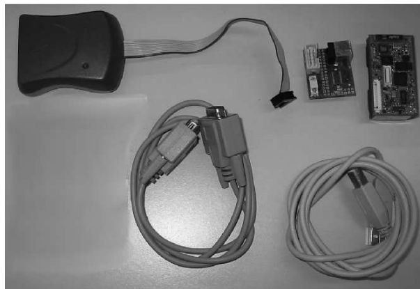
Figure 2: The BTnode development kit. The minimal set of tools consists of the three items on the very right: a BTnode, a USB programming board, and a USB cable. Additionally, there are an ISP (In-System-Programmer) and a serial cable (left half).
