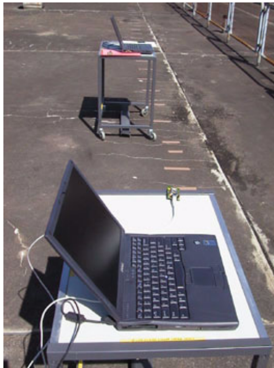
Picture: 2-6: Laptop on a trolley with the Bluetooth node attached
