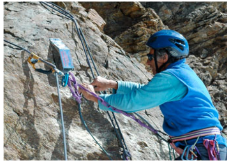
Fig. 2: The Permasense projects uses wireless sensor network technology to monitor permafrost and global warming in the Swiss alps
