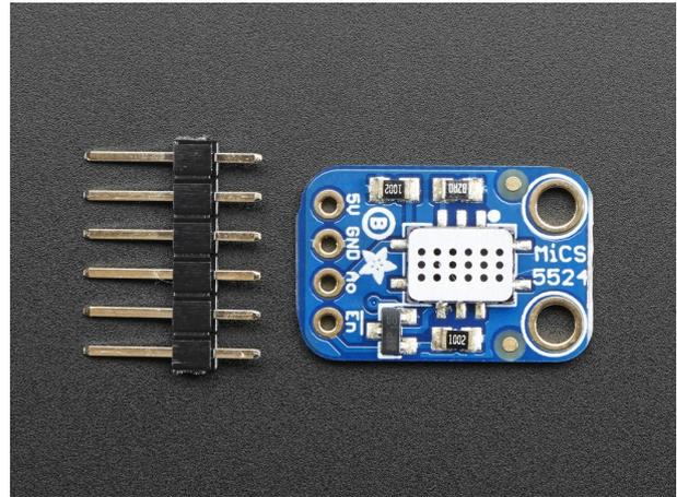
Figure 1: Breakout board of a popular metal-oxide air quality sensor.
