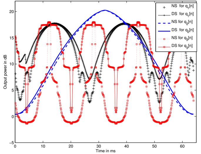
Fig. 2: Output power as a function of time for NS and conventional DS beamformers. Output powers have been calculated for 3 different nonstationary noises with  $q_1[n] = (|\cos(40\pi n/8000)| + 0.1)^2$ ,  $q_2[n] = e^{-2(0.004n-1)}(\frac{1}{2} + \frac{1}{2}\cos(32\pi(n-256)/8000) + 0.1)^2$  and  $q_3[n] = ((\sum_k \Pi(n/64 - 2k)) + 0.1)^2$ , respectively. In  $q_3[n]$ ,  $\Pi(t)$  is a rectangular function that is equal to 1 for  $0 \leq t \leq 1$  and 0 otherwise.
