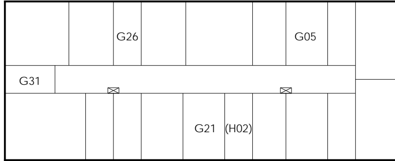
Figure 2. Floor plan of the building where the described system evaluation has been carried out. Base station positions are indicated by crosses; room H02 is on the next higher floor.
