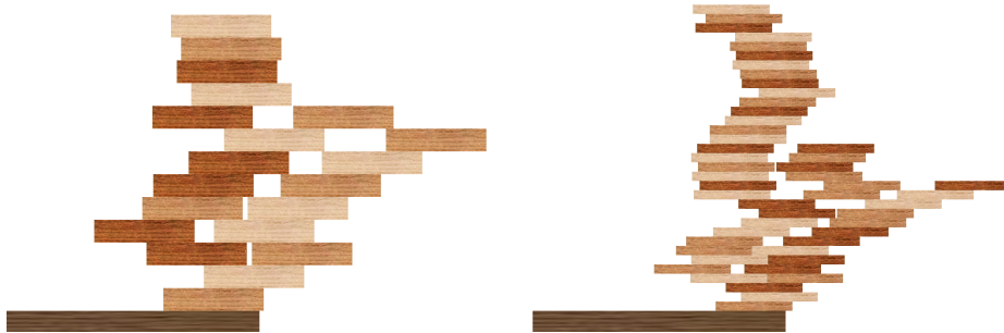
Fig. 7. Best stacks identified, for 20 blocks on the left (overhang = 2.275) and for 50 blocks on the right (overhang = 2.97)
