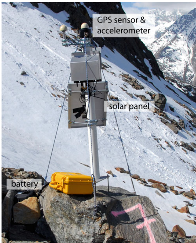
Fig. 4 GPS station at position DI7, on the destabilized tongue of the Dirru rock glacier. Station DI7 includes a logger, two inclinometers and a prototype online sensor, all mounted on the same mast. Energy supply is given by a photovoltaic energy harvesting system
