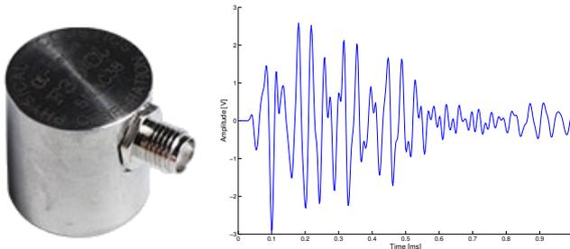
Figure 1: Acoustic emission sensor with an example of its analog output signal.
