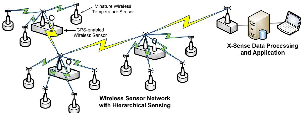
Fig. 1: Hierarchical sensing system concept.
