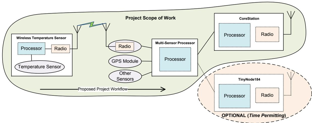
Fig. 2: System architecture and project scope of work.
