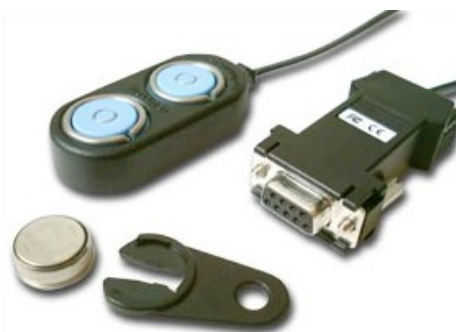
Figure 1. Coin-sized iButton device and 1-wire device programmer. The maximum diameter of an iButton device is 17.35 mm, the maximum height is 5.89 mm.
