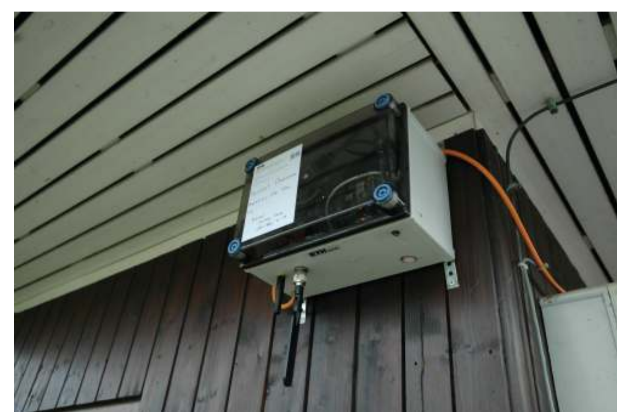
OpenSense node placed next to the NABEL station Duebendorf for initial calibration
