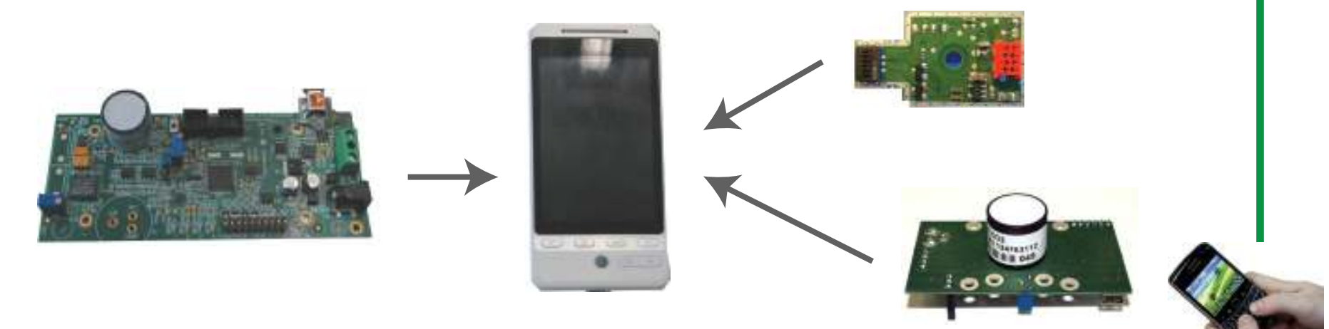
Smart phone controls several gas sensors
