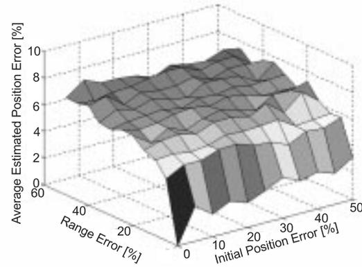
Fig. 5. Refinement, 10 nodes, 4 anchor nodes, 25 iterations
