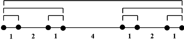
Fig. 9. A recursive arrangement of eight nodes on a horizontal line. The labels indicate distances.
