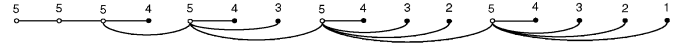
Fig. 14. The interference of the exponential node chain—shown in a logarithmic scale—is bounded by O(\sqrt{n}) by the topology control algorithm \mathcal{A}_{\text{exp}} . Only hubs (hollow points) interfere with the leftmost node. For clarity of representation, some edges are depicted as curved arcs.
