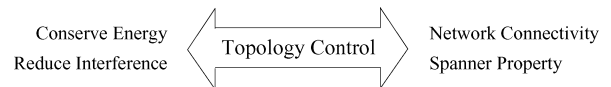
Fig. 1. Topology control constitutes a tradeoff between node energy conservation and network connectivity.
