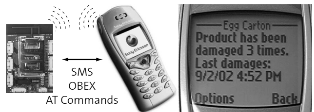
Figure 3. Product monitoring using BTnodes as smart tags and SMS via mobile phones
