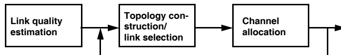
Fig. 2. Our algorithm to construct the network is incremental and subsequently involves link quality estimation, link selection and channel allocation.
