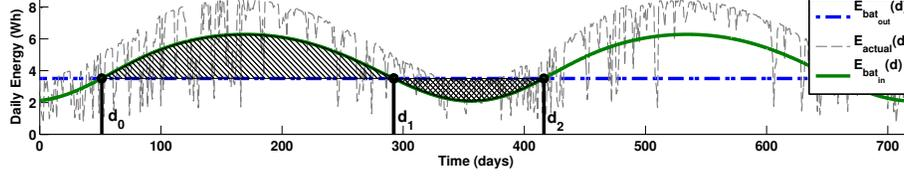
Figure 2: Actual ( $E_{actual}$ ), and modeled daily energy input ( $E_{bat_{in}}$ ) and output ( $E_{bat_{out}}$ ) for panel area  $A_{pv} = 0.02m^2$  over two years of the CA dataset (see Sec. 6.1). Surplus energy is indicated with the hatched area. The cross-hatched area shows the required battery capacity.
