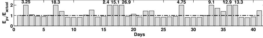
Figure 3: Ratio of total daily energy predicted with our approach ( $E_{pv}(d, \Omega = 0.51)$ ), and actual energy input ( $E_{actual}(d)$ ) for each day. Note: bars are capped at 2, and labeled with actual value.
