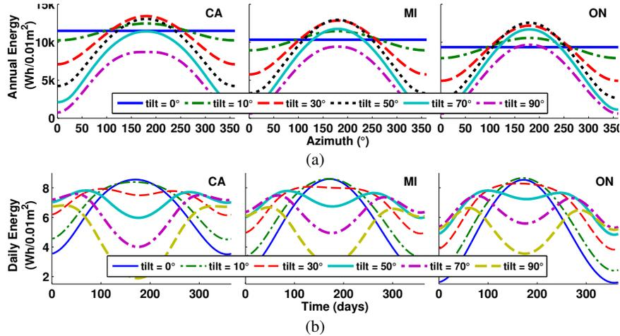
Figure 6: (a) Total *annual* energy incident with inclination angles from  $0^\circ$  to  $90^\circ$  as a function of azimuth angle. (b) Total *daily* energy incident over one year for inclination angles ranging from  $0^\circ$  to  $60^\circ$  ( $\tau = 0.1$ ,  $k = 0.3$ ,  $R = 0.3$ ,  $\eta_{pv} = 0.1$ ).
