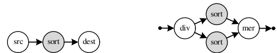
(a) Top-level process network of the quicksort algorithm. (b) Structural description of process “sort”.
