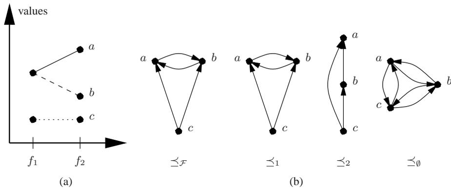
**Fig. 8.** (a) Parallel coordinates plot for an example with three solutions  $a$  (solid line),  $b$  (dashed), and  $c$  (dotted) and two objectives  $\mathcal{F} := \{f_1, f_2\}$  with no conflict according to Def. 8.  $\{f_1\}$  is nonconflicting with  $\mathcal{F}$  whereas  $\{f_2\}$  is weakly conflicting with  $\mathcal{F}$ . (b) shows the corresponding relation graphs of the involved relations  $\mathcal{F}' \subseteq \mathcal{F}$ .
