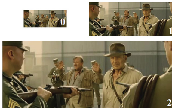
Fig. 1. Spatial scalability with three spatial layers. The resolution doubles with each layer.
